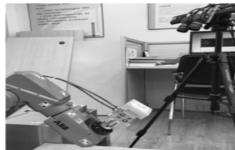
Figure 2. Positioning accuracy verification experiment The method used in this paper is that the claws at the end of the robot grab objects and move them to different postures. The experiment process is shown in Figure 2, and 10 sets of images are collected. The experimental task is to identify, locate and capture multiple objects in the scene. According to the end pose
